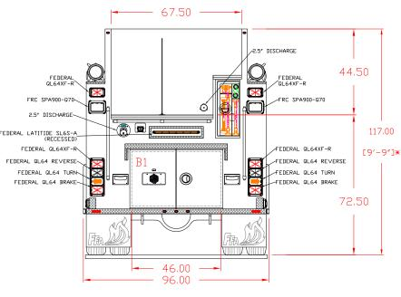
10-24-23 APPROVAL (AN) \*HEIGHT COULD VARY +/- 2" BASED ON LOADING OF VEHICLE
