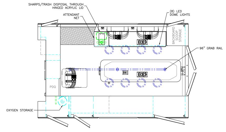
$\star$  (1) ANTENNA BASE LOCATED OUTBOARD OF DOME LIGHT WITH COAX SERVICE LOOP
