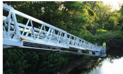
Operate at negative elevations up to -12° reaching over 11' below street level
