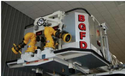
Twin monitors are available both manual, 1 manual and 1 electric or both electric
