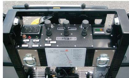
Platform controls are located front-center, giving the operator the best view when positioning the bucket
