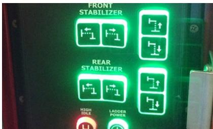
Our outrigger controls are waterproof, rubberized push buttons, which are function illuminated for fast setup
