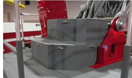
The rotation drive is under the turntable step with easy transition from the turntable to the aerial ladder
