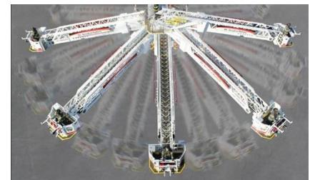
Operate on ground only 33' from apparatus with 240° of rotation at -12° reachaching 9' below street level extended
