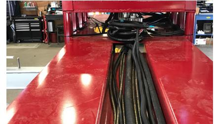
The top of the torque box has a recessed channel to accommodate wiring and hydraulic lines
