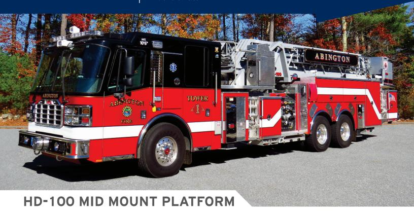
The Ferrara HD-100 Mid Mount Platform is our popular low profile, low travel height 100' platform. With a standard height of only 10' 9", the HD-100 MMP fits in nearly any fire house. Able to be designed as a quint or traditional truck, the 5-section aerial platform features Ferrara's impressive horizontal reach, able to reach a 7th floor and overcome over 70' of set-back. Operating off an overpass or bridge, the HD-100 can extend over 11' below street level and reach 96' from the turntable.
