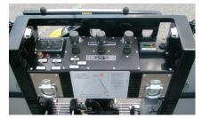
Platform controls are located frontcenter, giving the operator the best view when positioning the bucket
