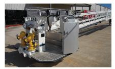
Ferrara's optional rope rescue/lifting arm also doubles as a temporary stokes mount
