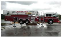
Forward stabilizers are directly behind the cab and support the weight of the cab and chassis
