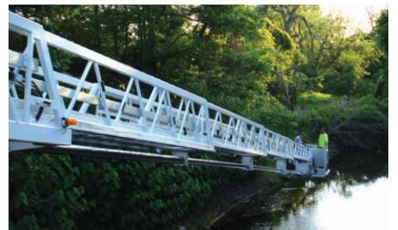
Operate at negative elevations up to -12° reaching over 11' below street level
