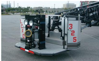
Bi-fold opening gates provide up to a 24" wide opening, wide enough to accommodate a stair chair
