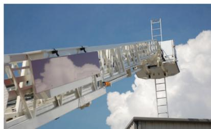
Our optional parapet roof ladder bracket allows you to safely access a parapet roof from our platform
