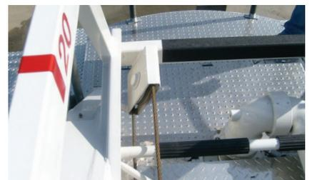
All sheaves are fully enclosed, so PPE or other gear won't get caught between the cable and pulley
