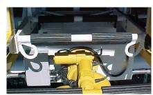
Standard pair of load lifting eyes at the ladder tip are rated at 500lbs as a pair for rescue capability
