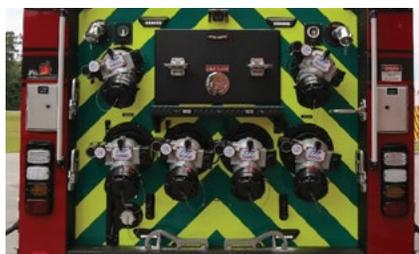
Rear Inlet / Outlet Connections
