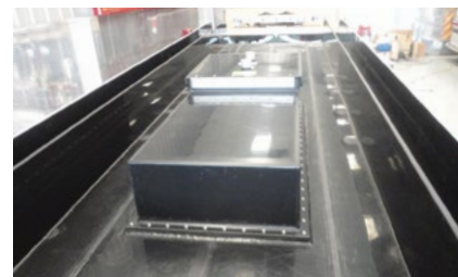
Tank integral hose bed storage areas
