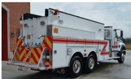
Painted poly wet side configuration tanks
