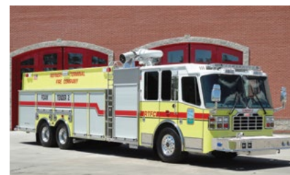
4000 gallon foam tenders with manifold system, foam system, and 8000 gpm monitor
