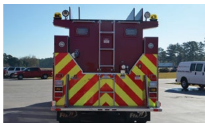
Multiple discharge and direct tank fill options as well as hosebed access ladders
