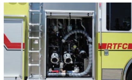
Manifold/monitor modules available with foam proportioning systems
