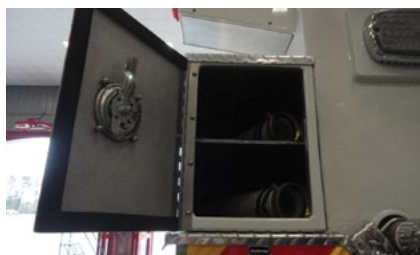
Foam suction hose storage compartments
