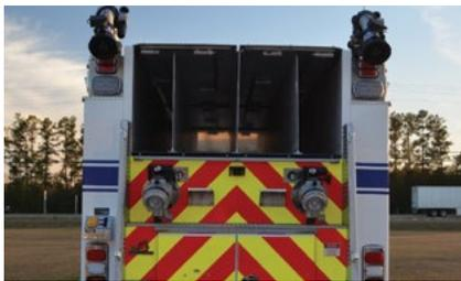
Hosebed Fall Suppression Systems with Electric Over Hydraulic Door Lift Struts
