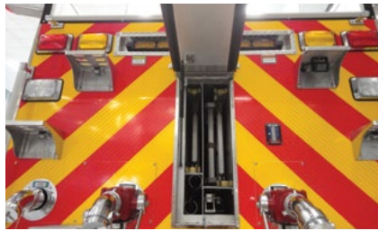
Enclosed through-the-tank storage
