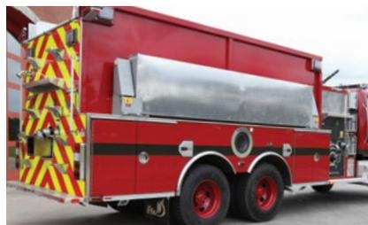
Hydraulic portable tank rack
