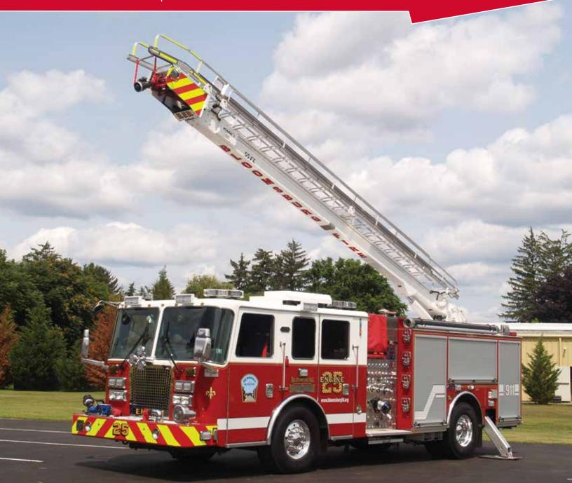
The KME AerialCat™ FireStix is versatile with minimum setup time to maximize your firefighting response and offers the best of both a pumper and ladder truck. It can be rated as a pumper or aerial. The FireStix is available on either a commercial or custom pumper chassis with a 500 lbs. tip load ladder. KME FireStix water towers are known for their maneuverability with the shortest wheelbases, overall lengths and lowest travel heights in the industry.
